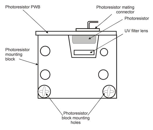
Figure 28. Photoresistor Assembly for Direct View (I300M)
